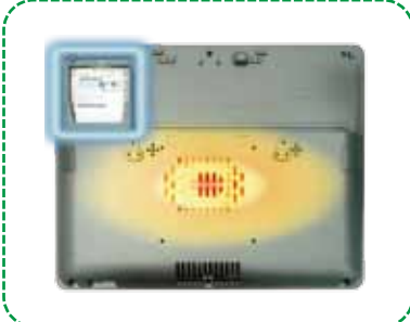
HDD isolated from main heat source on mother board
