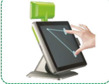
Projected capacitive technology (PCT) & multi-touch function
